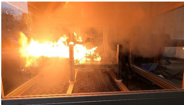
Figure 10: Jet flame during the thermal runaway of a 10,000 mAh pouch cell in the demonstrator (Janßen & Saupe 2023)
