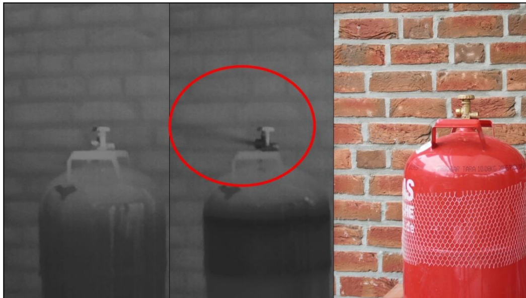
Figure 11: Simple gas detection using a DJI Mavic 2 Enterprise Advanced drone. Left = temperature of the cylinder in normal condition, center = cooling of the air and valve during gas leakage visible in the thermal infrared image (dark), right = gas leakage not visible in the simultaneously recorded RGB video.
