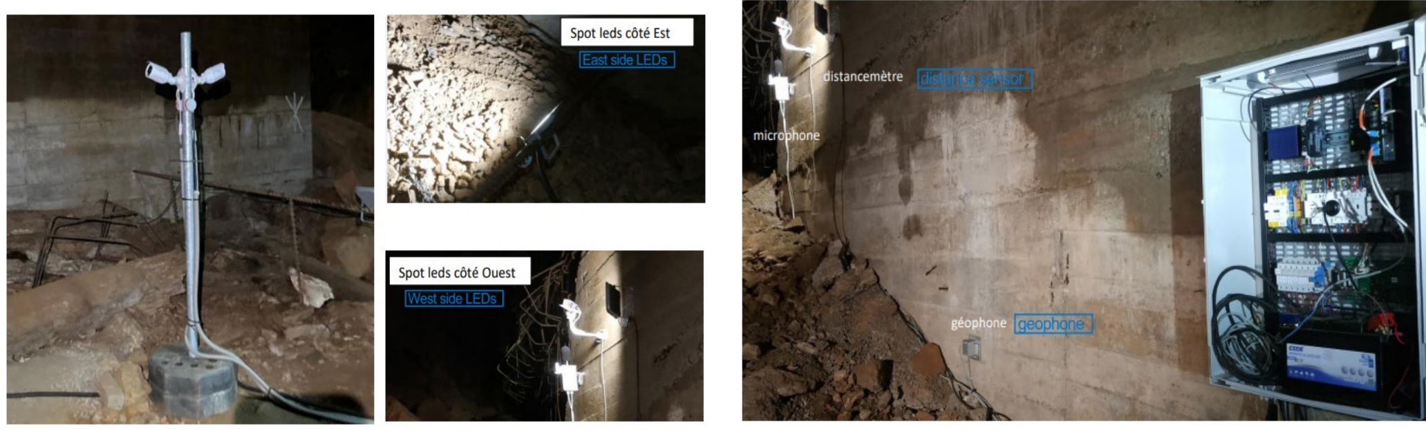
Figure 5: The seismic sensor system was installed in Thil. [2]
