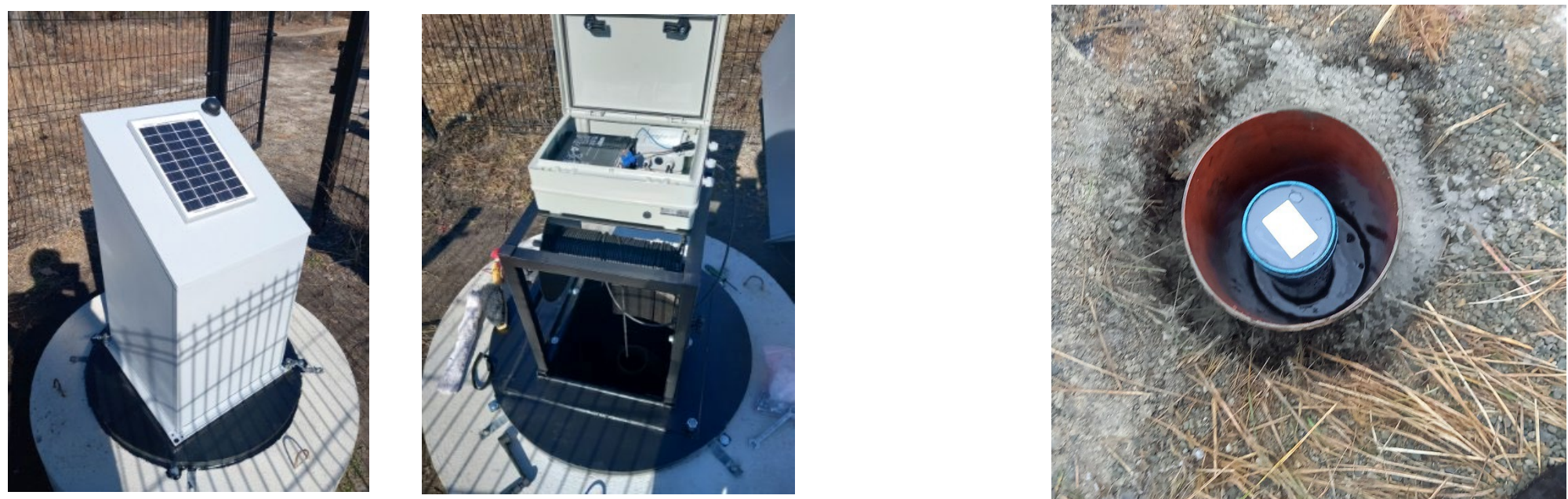
Figure 6: The piezometer with automatic measurement capabilities tracks changes in groundwater table, in Kazimierz. [3]
